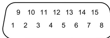
**Figure 10-1: Data Port Pin Layout**
