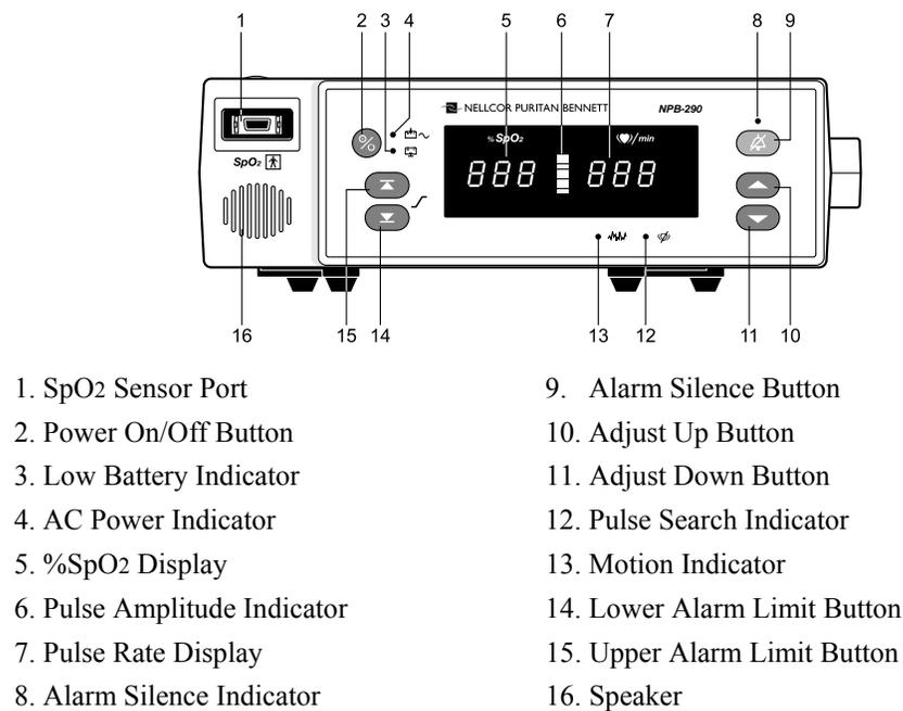
**Figure 1-1: NPB-290 Front Panel**
