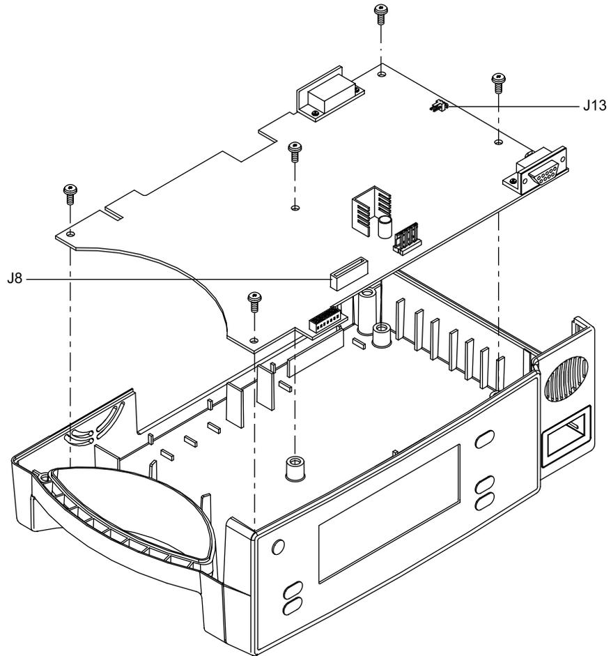
Figure 6-9: User Interface PCB
