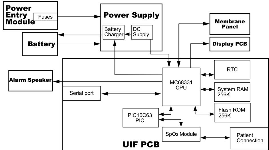
Figure 11-2: NPB-290 Functional Block Diagram
