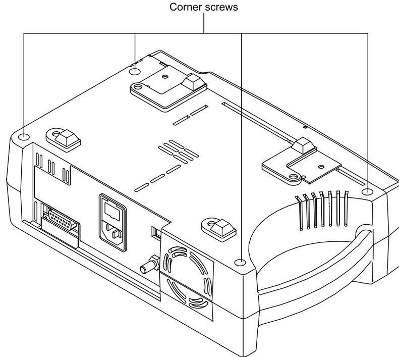
**Figure 6-2: NPB-290 Corner Screws**
