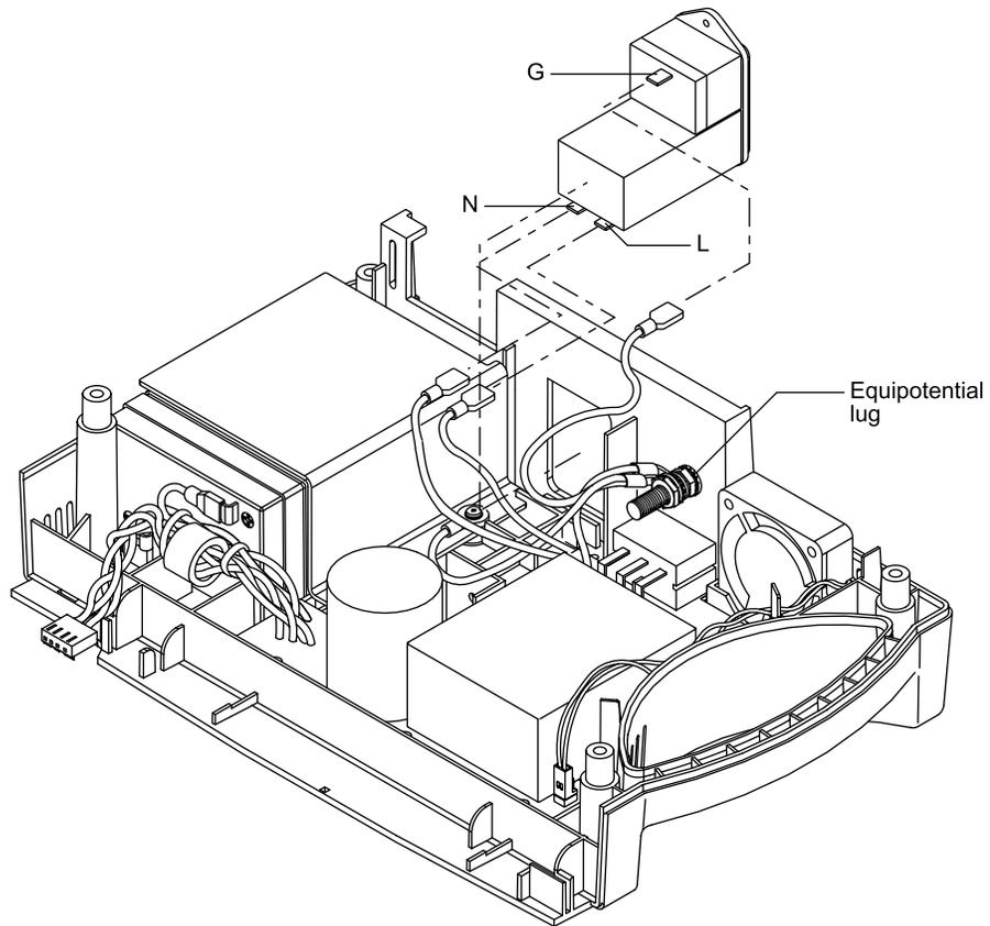
**Figure 6-5: Power Entry Module**
