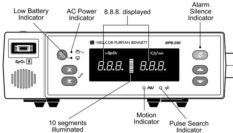
**Figure 3-2: Power-On Self-Test Display**
