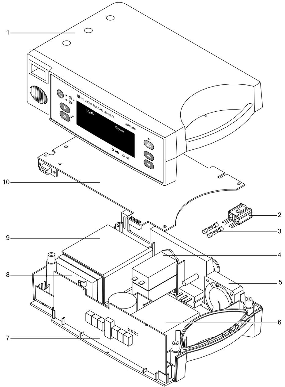
Figure 7-1: NPB-290 Exploded View
