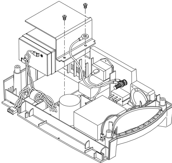
Figure 6-4: Battery Removal
