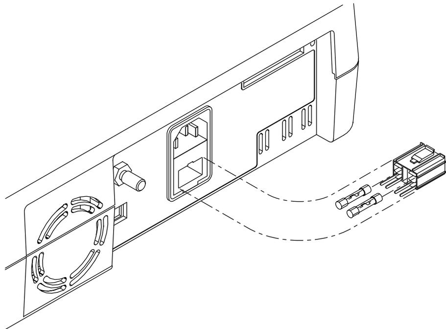
**Figure 6-1: Fuse Removal**
